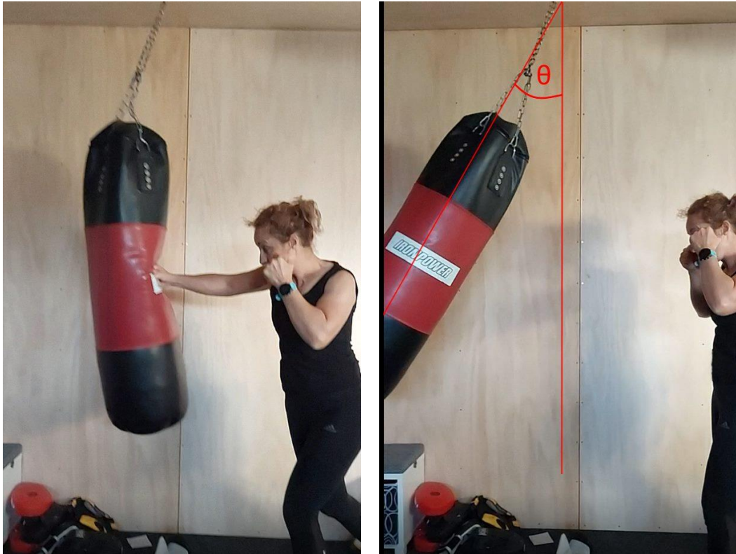
Figure 1. Screenshots of a video taken during a gyaku tsuki into a punching bag: (a) maximum deformation of bag and (b) peak height/angle of bag.
